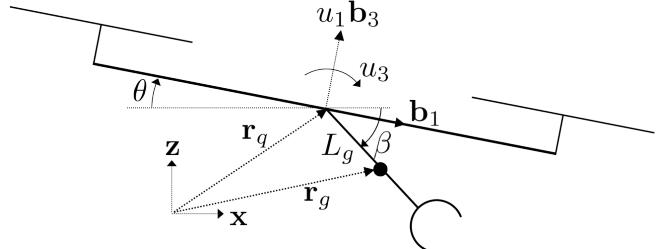
Fig. 1. The quadrotor has control inputs  $u_1$  in the  $b_3$  direction and  $u_3$  as a moment about the axis into the page ( $b_2$ ). The gripper forms the angle  $\beta$  with the horizontal and its center of mass is located a distance  $L_g$  away from the quadrotor’s center of mass.
