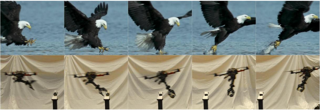
Fig. 2. A still image comparison between the eagle (extracted from [3]) and the quadrotor for a trajectory with the quadrotor moving at 3 m/s (9 body lengths / second) at pickup. See [10] for a video of the grasping.
