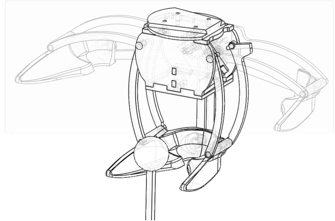
FIGURE 2. AN EARLY PROTOTYPE GRIPPER THAT COULD BE USED WITH SPHERICAL TARGETS. UNFORTUNATELY, THE GRIPPER WAS NOT PARTICULARLY SUCCESSFUL IN RETRIEVING NON SPHERICAL OBJECTS. THE GRIPPER IS SHOWN IN ITS OPEN (SHADED) AND CLOSED (SOLID) CONFIGURATIONS.
